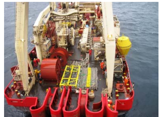
▲ Mattresses on Fu Hai Deck
